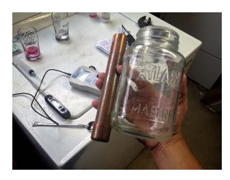
If you have the means then go ahead and sweat the pipe and solder the cap onto the pipe. You can also get away without soldering as was in my case since the fit was very snug. It hasn't leaked yet™.
